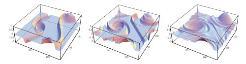
FIGURE 3.4. The time evolution of vorticity in two-dimensional inviscid Euler equations (2.8b) using a central difference scheme [137] computed at t = 4,6 and t = 10.
