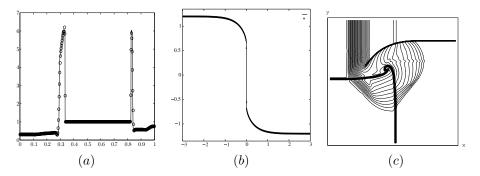
FIGURE 3.8. Numerical solution using FV central schemes. (a) Density of compressible Euler equations computed at t=0.01 using a central discontinuous Galerkin method [142]. (b) Saturating dissipation,  $w_t + f(w)_x = \left(w_x/\sqrt{1+w_x^2}\right)_x$  [126]. (c) Density contours of two-dimensional Riemann problem (without a Riemann solver).
